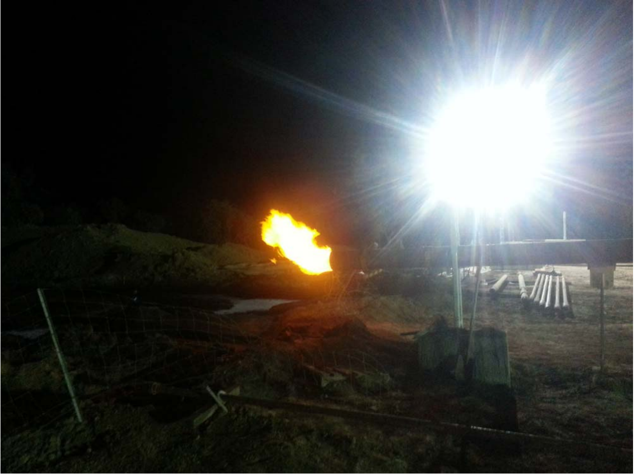
Figure 2 - Flare observed upon reopening the Egiliabria 2 vertical well after brief shut in
