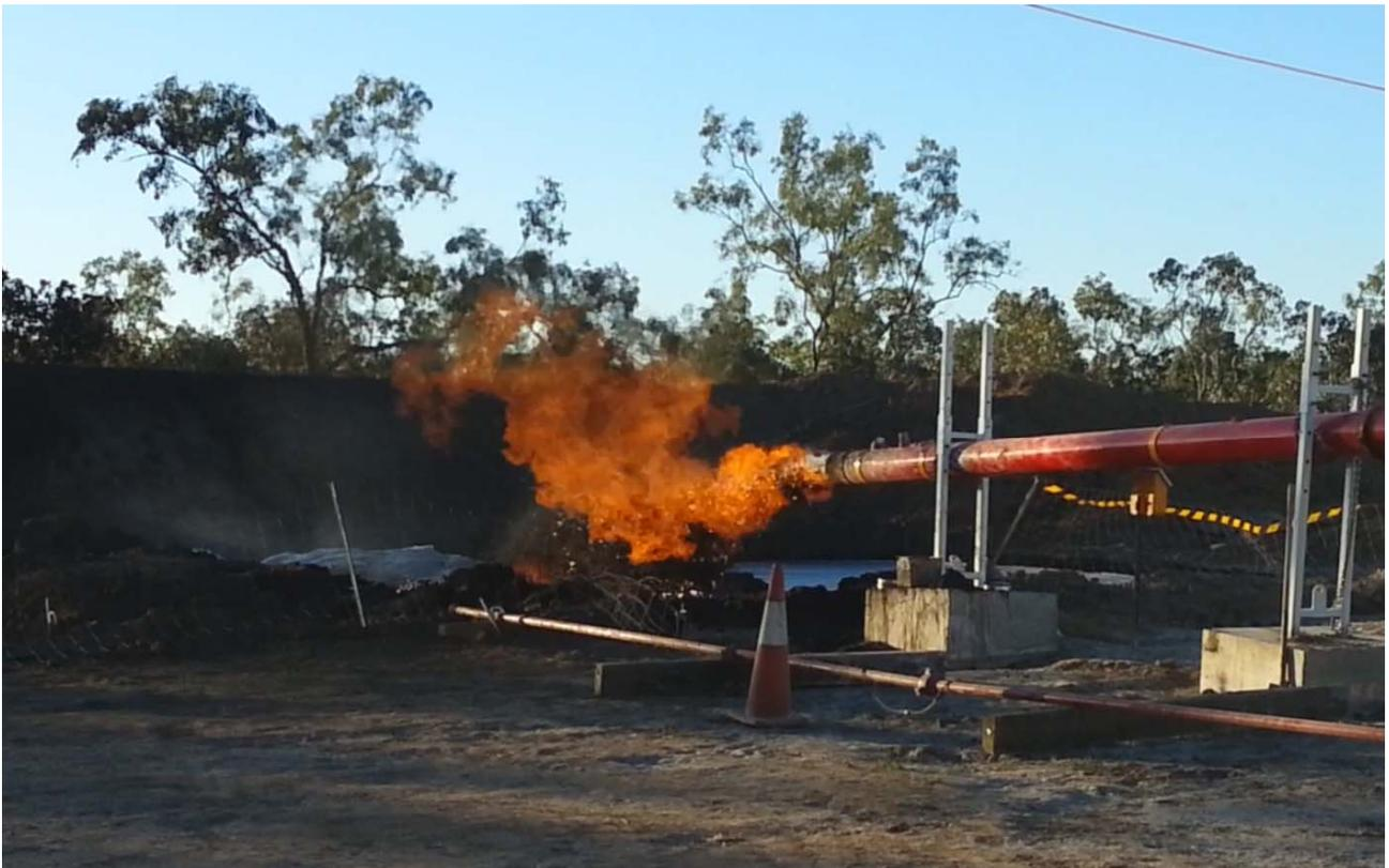
**Figure 1 - Flare observed upon reopening the Egiliabria 2 vertical well after 4 hour shut in**
