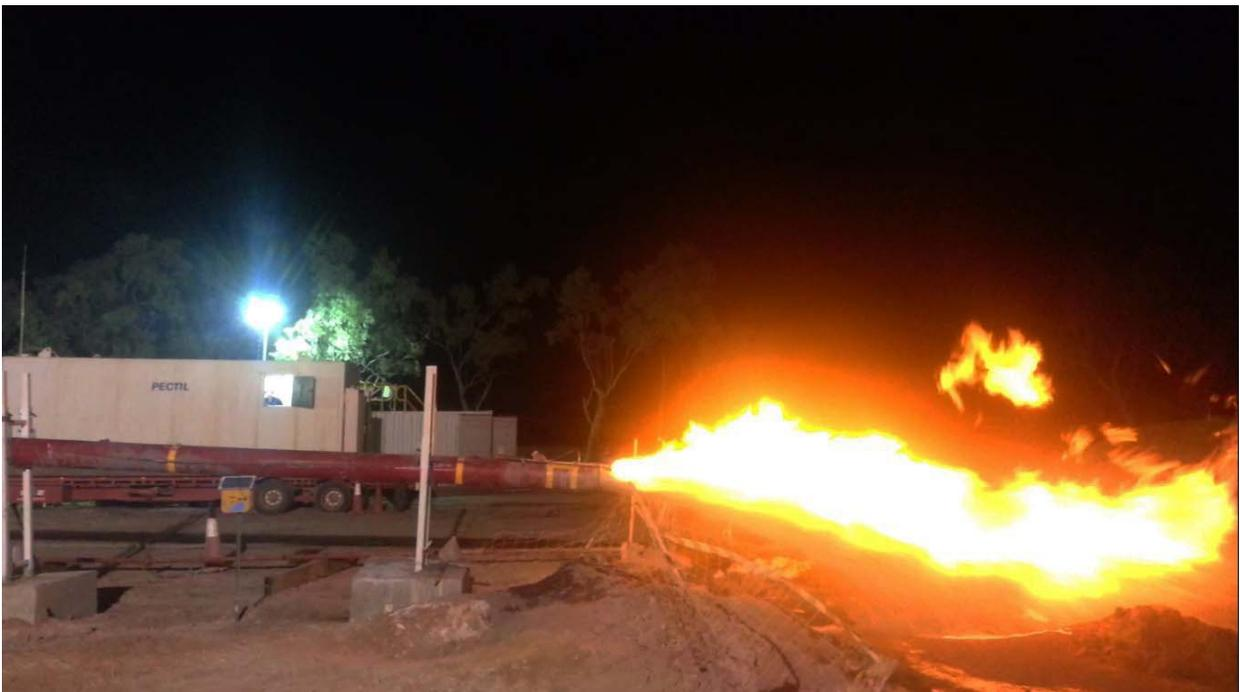
**Figure 1 - Flare observed on 3 July during bit changeout from previous gas zone encountered at 1519 metres in the Egilabria 2 well.**
