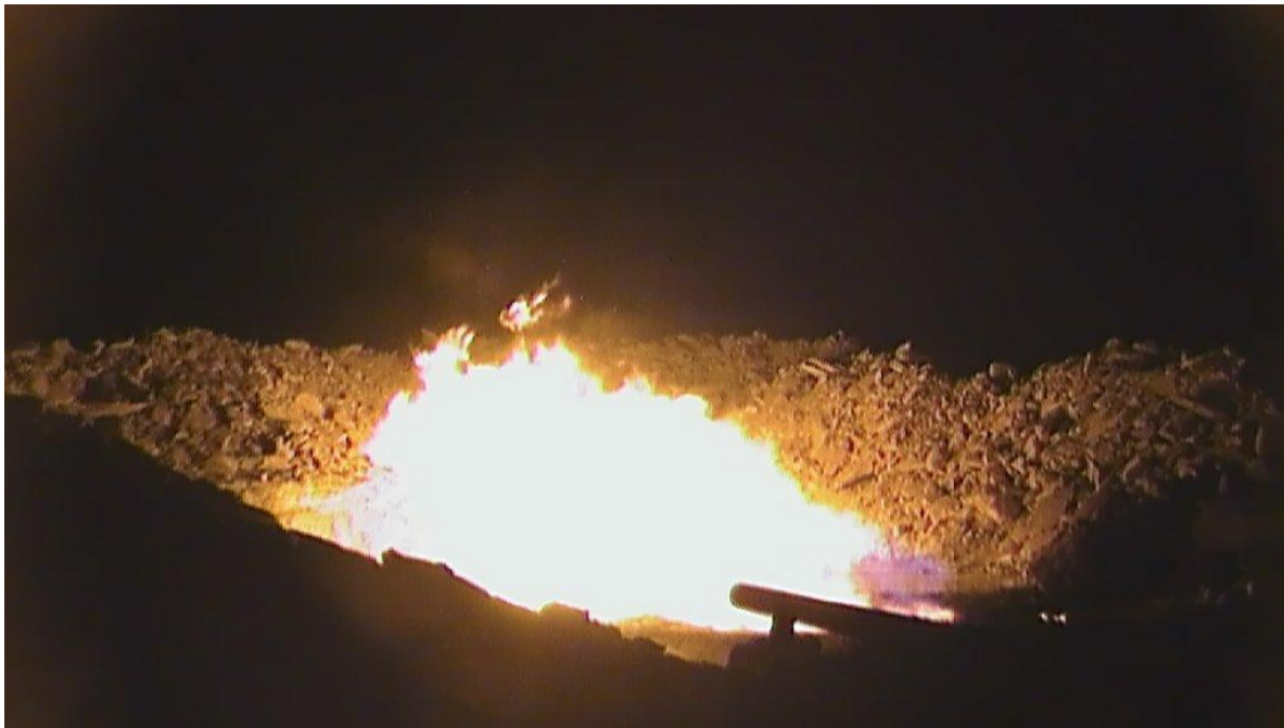
Figure 3: Gas Flare during Testing at Glyde #1 Lateral Well Measured Well Depth of circa 670m
