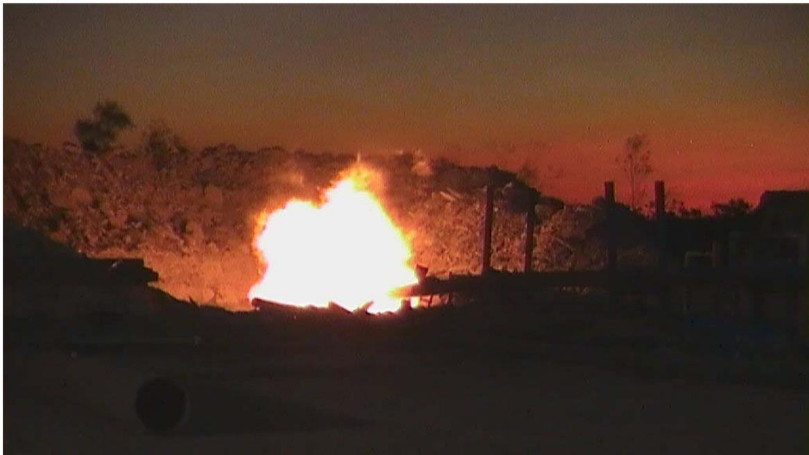
**Figure 3: Gas Flare during Drilling with Compressed Air at Glyde #1 Lateral Well
